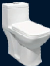
MIA 7022 P & 9 One Piece Toilet - Washdown Size:- 635 X 340 X 670 mm Dual Flush; Soft Close seat cover P' Trap - 300 mm S' Trap - 225 mm
